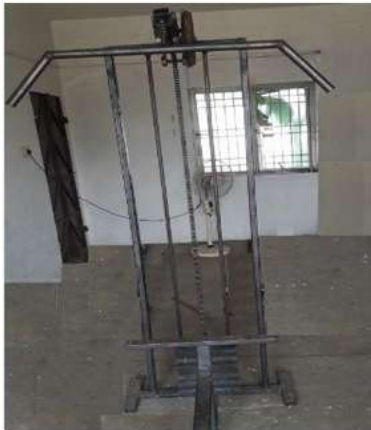
Fig. 8 Lat pull down machine for power generation
